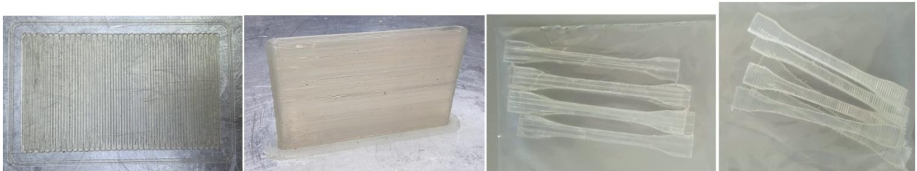
Figure 2.7 - Horizontal and vertical plates of size 150x90x2 mm (first two on the right, respectively), and examples of specimens for tensile test in the XY orientation and XZ orientation (last two on the left, respectively)
