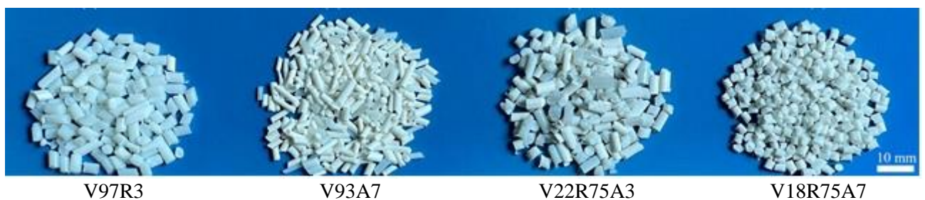
Figure 2.4 - Pellets from different composites produced for this thesis. The letter V stands for virgin polylactide, R - for polylactide debris, and A for titanium dioxide nanoparticles. The number to the right of the letter indicates the percentage of each material in the mixture
