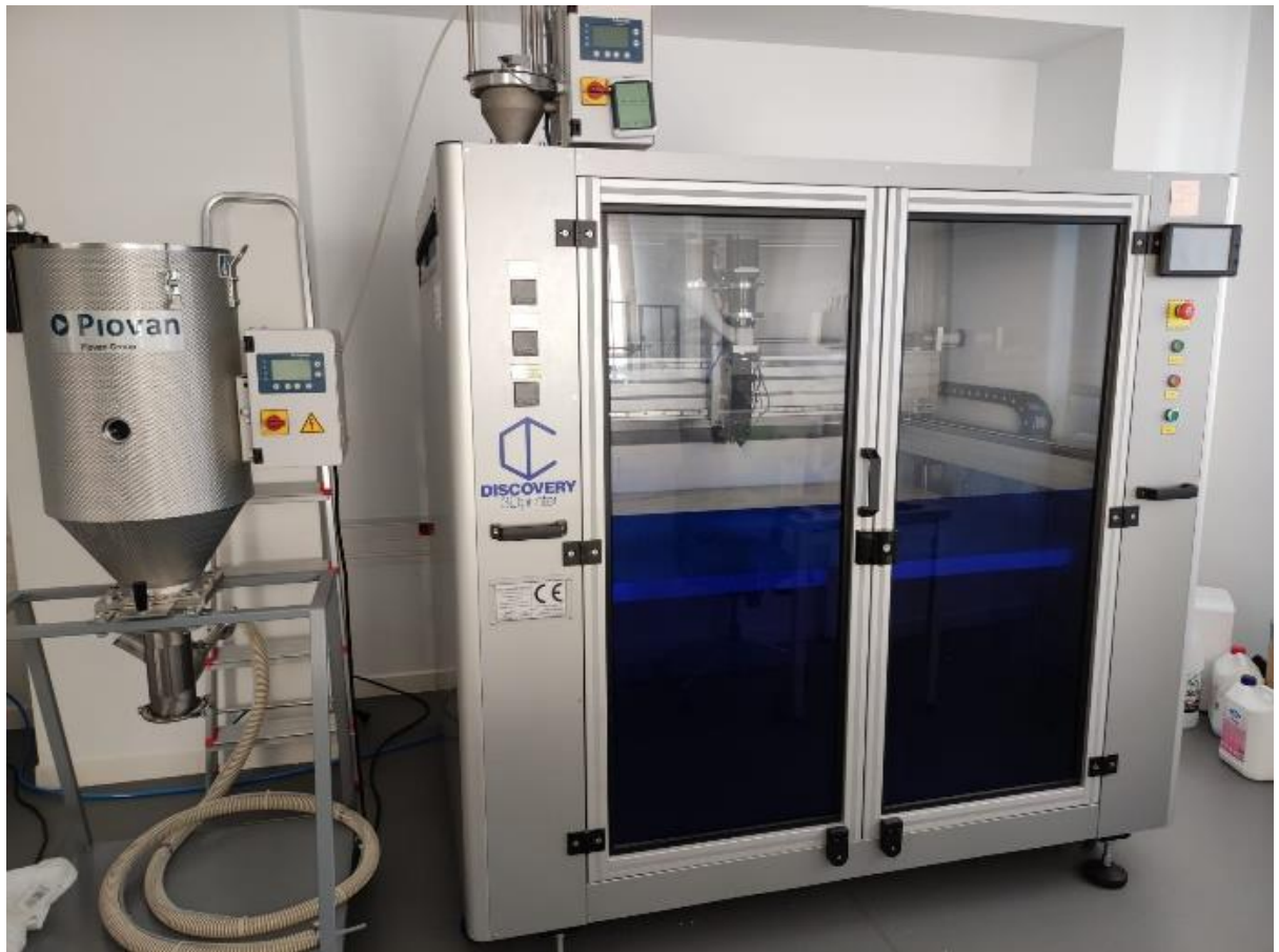
Figure 2.5 - Discovery 3D Granza printer (right) and Piovan dehumidifying dryer (left)
